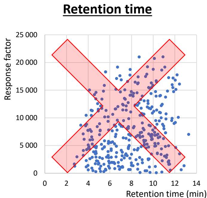
Figure 2: Response factor versus retention time for 351 compounds
